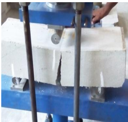
Figure 1 Flexural strength Test
