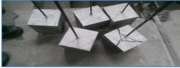
Figure 4 Cubes After cured in Autoclave
